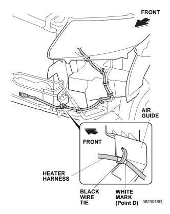
28. With the help of an assistant, route the heater harness through the front bumper in the area shown, and reinstall the front bumper.
