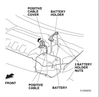
11. Remove the battery cover, battery, and battery tray.
